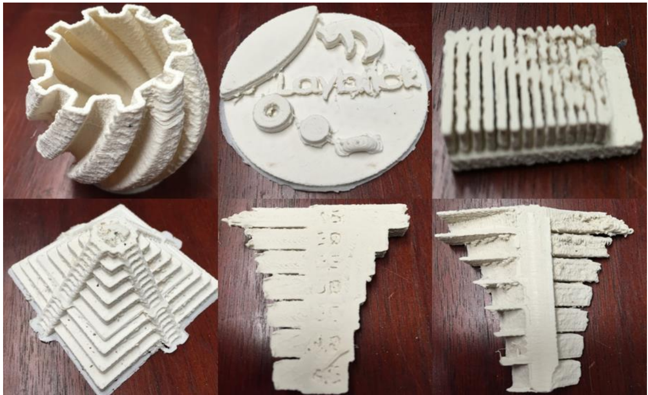
Images (Left to right, top to bottom): Single walled vase, Artifact/Feature size test, Retraction/Feature size test, arch, top of overhang test, bottom of overhang test.
